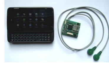
Figure 8. The Dandelion prototype hardware, based on Nokia N900 smartphone (left) and Rice Orbit body sensor (right)
